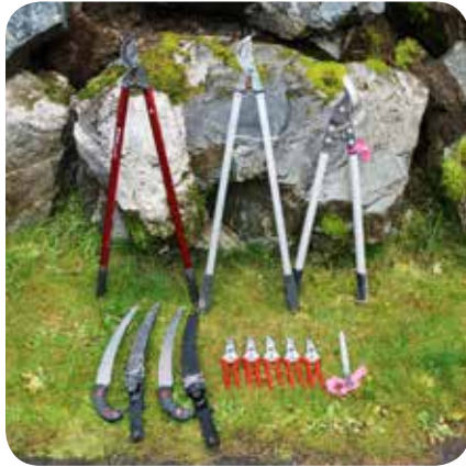
Tools for cutting woody invasive species include loppers, pruning saws, secateurs and a file for keeping everything sharp. Photo: D. Polster
