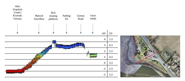
Figure 6 - Typical elevation profile of Dyke Road Park. Red line in the righthand map image shows the location of the profile across the site. The horizontal axis of the lefthand profile panel is compressed; total profile length is approximately 120 m. Elevations are approximate. Data source: City of Courtenay LiDAR (2012).
